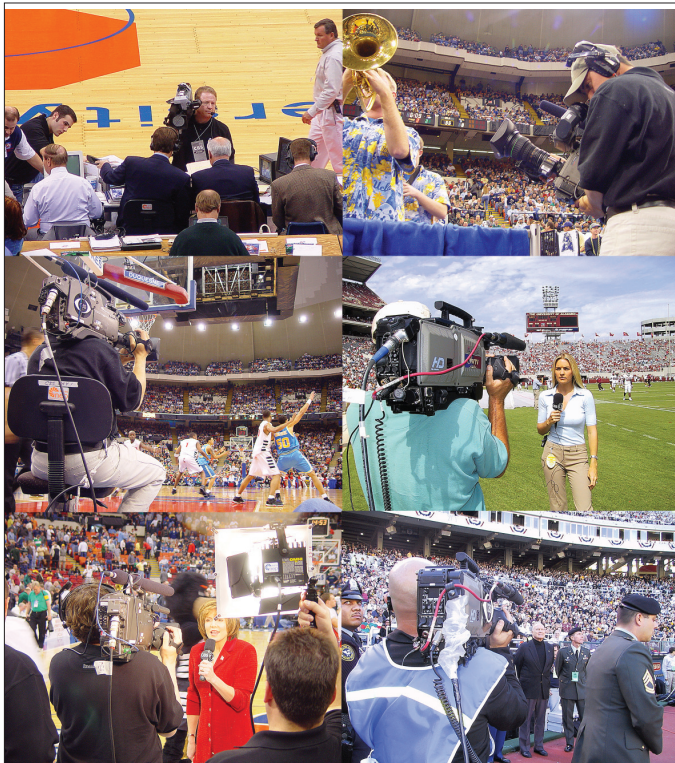
Figure 4.28 Today's cameras, tethered to the truck via triax or RF link, can get anywhere the cameraman can.
