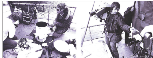
Figure 4.21 By the mid-70s, cameras were portable enough to sit on a person's shoulder and to fit in small diving bells (still with a tether to the CCU), as seen in these two photos. On the left, a Norelco PCP-90 is disassembled and checked after the diving bell sprung a leak. On the right, a cameraman with a TKP-46 on his shoulder points to a PCP-90. (Source: Jerry Hughes)
